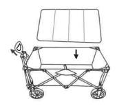
Put the cushion into cart and hold the handle to lift up
