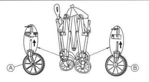
2. Press the black button to install the front and back wheels
