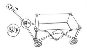
4. Press the center button to fold the handle
